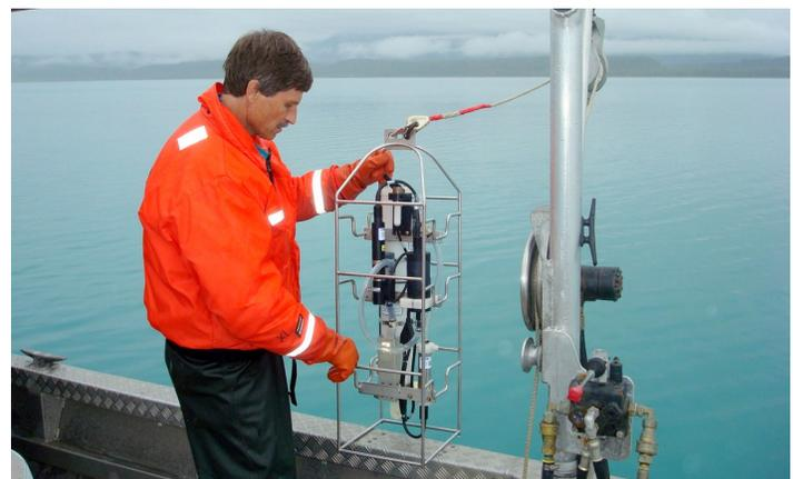
A National Park Service researcher deploys a CTD instrument (Conductivity-Temperature-Depth) to measure water column characteristics at a sampling station in Glacier Bay. This monitoring effort aims to document interannual and seasonal variation in physical oceanographic conditions in Glacier Bay and to provide a baseline oceanographic dataset that can be used by researchers to understand spatial and temporal variation in the biological productivity of Glacier Bay.
